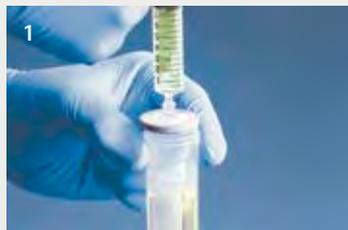
1. Stable fit of the filter on a 50 ml centrifuge tube
