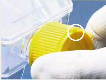
VENT position at 12 o'clock = gas exchange
